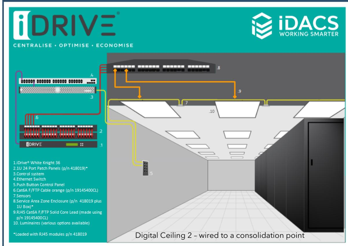
Category 6A cabling must be used for connectivity, as the maximum current carrying capacity per cable core is 500mA thus allowing up to 2A forward current to be used with the attached LED luminaires.
