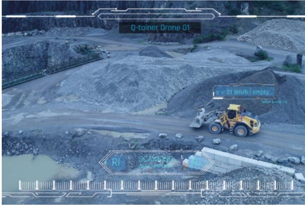
Using drone images among other things the system records movement profiles and load sizes of the construction machinery in the RCR.
